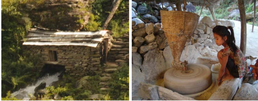
Figure 2.7: Ghatta house (left) and Ghatta (right): Traditional water mill for grinding grain made in local level near Sunkoshi River, whose Nepali name is Ghatta, the massive runner stone disc. Water is diverted from a stream or river and flows down a rectangular chute called dunde , towards the Ghattas turbine, called Madani . The vertical shaft of the turbine runs in the vertical direction through the floor of the ghatta house and horizontally rotates the upper runner stone of a pair of grinding stones. Grain is stored above the runner stone in the hanging silo and exits out through a feeder mechanism at the bottom of the silo in a control manner into a central hole of the upper runner stone, and is then ground between the pair of stones (Photo: Field excursion during the symposium, MGDA-11).
